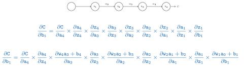
$$\frac{\partial C}{\partial b_{1}} = \frac{\partial C}{\partial a_{4}} \times \sigma^{'}(\mathbf{z}_{4}) \times w_{4} \times \sigma^{'}(\mathbf{z}_{3}) \times w_{3} \times \sigma^{'}(\mathbf{z}_{2}) \times \times w_{2} \times \sigma^{'}(\mathbf{z}_{1}) \times \mathbf{1}$$
